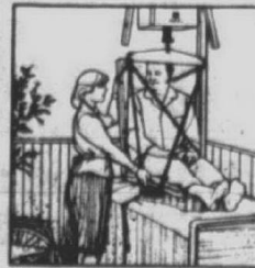
The lift motor automatically raises and positions the patient into a sitting position before transfer to a wheelchair.
