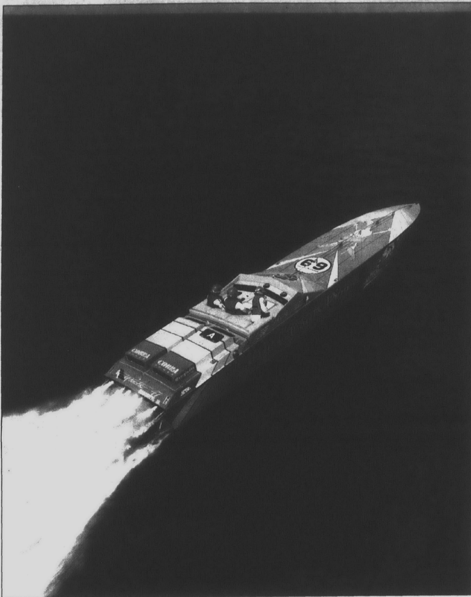
Peter Markey takes "Pan-Pan" along for a ride in his 47-foot, three-supercharged engine, 3,300-horsepower, 17,000-pound Deep-V Apache Superboat.
